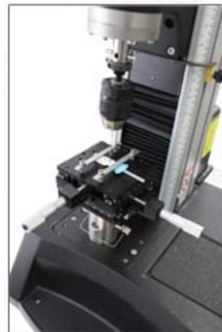
The combination of proper grip/fixture selection, consistent specimen placement, and minimizing offset loading effects on the load cell will help minimize the effects of side loading, ultimately reducing variation in results. Since the solution varies depending on your application, [contact](#) our Application Engineers for assistance.
